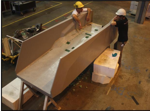
Figure 1.19: The scaled hull.
