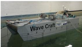
The active control of the air cushion has been confirmed in model testing.
