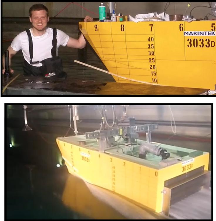
Figure 1.22: Resistance and drag tests in calm water performed in the Ship Model Tank.
