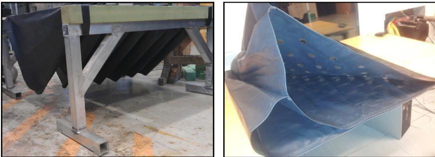
Figure 1.20: The scaled flexible seals.
