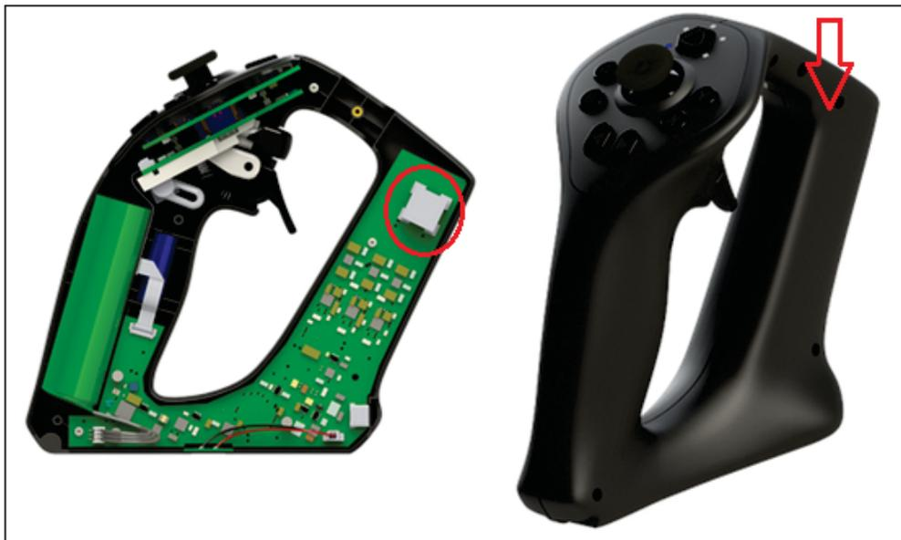
Figure 1.2: **STEM-controller:** The controller's electromagnetic tracker is placed as shown in red. Image from (Kickstarter: Sixense STEM, 2014).
