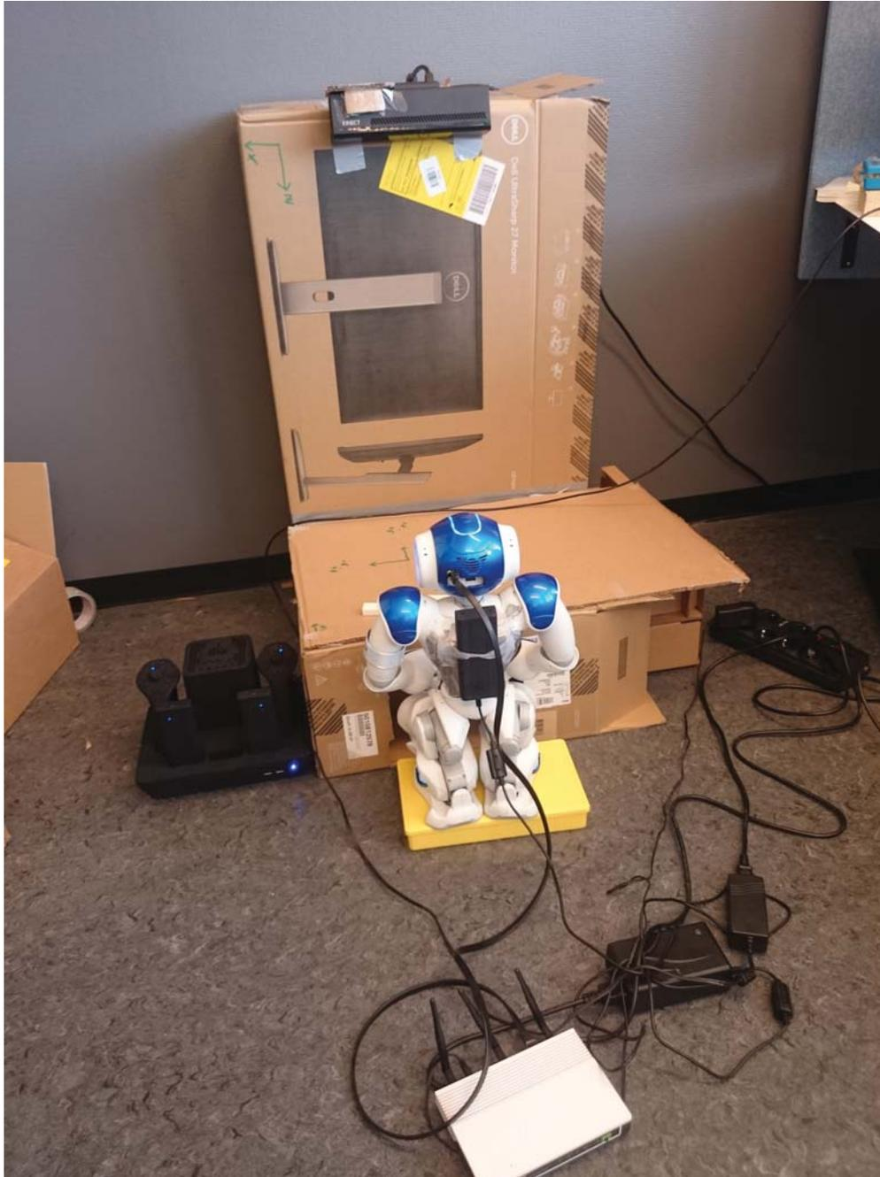
Figure 3.20: **Summer lab:** Here is the complete system from the summer project. The rig is made of cardboard because of Sixense STEM's metal sensitivity, and the robot is connected to the Internet through a cable because of the WiFi-sensitivity.
