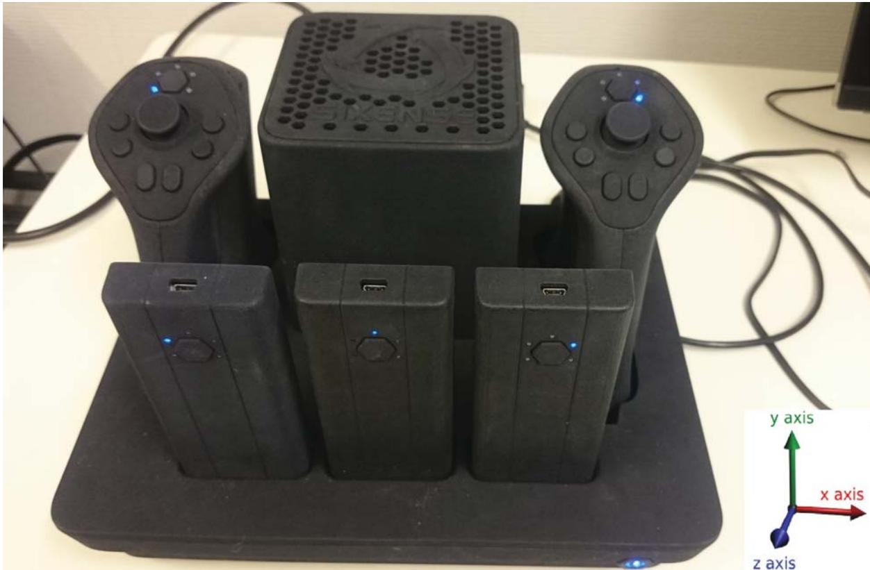
Figure 3.6: **STEM coordinates:** The coordinate system that the STEM-trackers follow are defined like shown in this figure, which is differently from the robot's coordinate system. Picture taken from (Evjemo, 2016)
