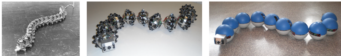
Figure 1.1: Selection of snake robots (from left to right: ACM III [Hir93], Kulko [LPSG12b], and Wheeko [LPSG12a]).
