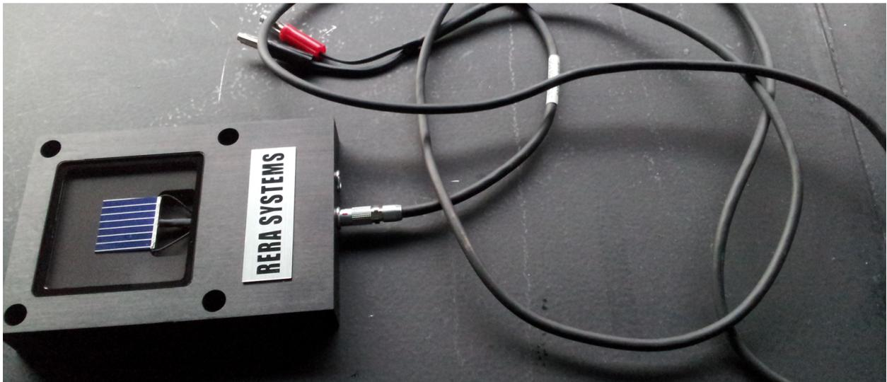
Figure 6.8: Photo of Rera Systems photovoltaic reference cell.
