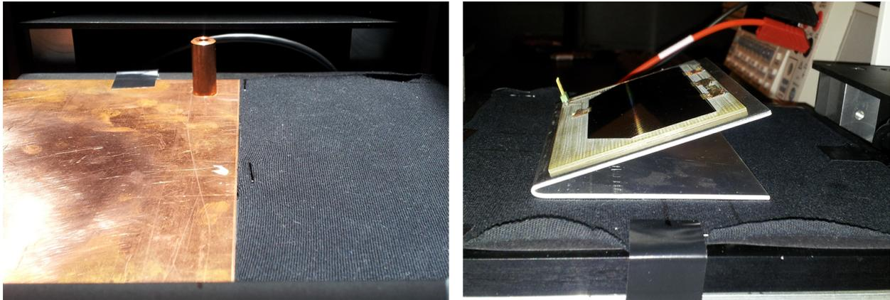
Figure 6.27: Photos showing the replacement work plane surface with lower reflectivity.
