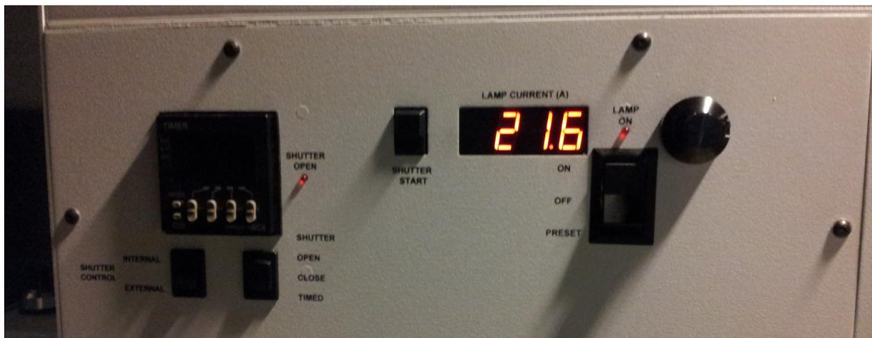
Figure 6.3: Photo of solar simulator control panel
