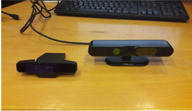
There were several concerns when selecting a 3D sensor. Firstly our inspection planning algorithm assumes data as a continuous stream with a sensor capturing depth in a cone. Thus sensors using time of flight, projected grids or stereo camera solutions are the most viable.
