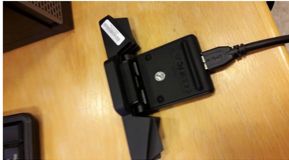
To attach a custom mount to the ur5 first a base is needed to attach to the wrist link. To this end SINTEF had a model of a cap that would fit the end effector forming a nice base. The endeffector is made by combining this with a mount for the camera.
