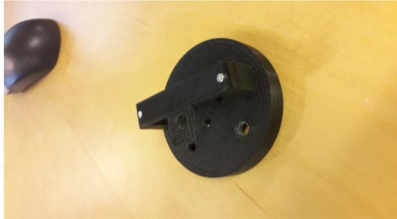
Measurements on the end effector places the center of the camera box approximately 4.5 cm out and 3.5 cm up from the end effector link.
