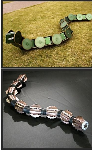
Figure 1.9: The snake robot ACM R3 (above) developed at Tokyo Institute of Technology. The robot is covered with passive wheels. **Image source:** [17]. The snake robot ACM R5 (below) developed at Tokyo Institute of Technology. The robot is covered by passive wheels and can swim under water. **Image source:** [18]
