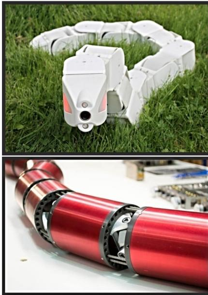
Figure 1.10: The snake robot Mamba (above) developed at NTNU. The robot is equipped with contact force sensors along its body. **Image Source:** [38]. The Snake Arm (below) without passive wheels, which is a holonomic mechanical system. **Image courtesy of OC Robotics, [www.ocrobotics.com](http://www.ocrobotics.com).**
