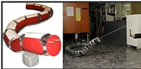
Figure 1.13: The snake robot Anna Konda developed at NTNU for fire fighting operations. Image source: [11]
