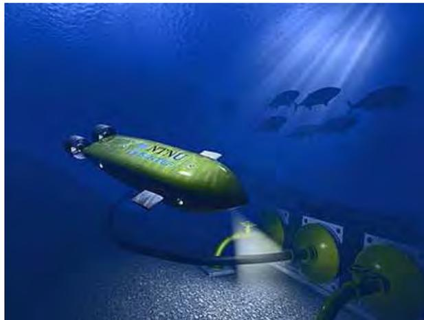
**Figure 8.2:** Illustration of the Munin AUV performing hovering inspection of an offshore oil and gas installation.
