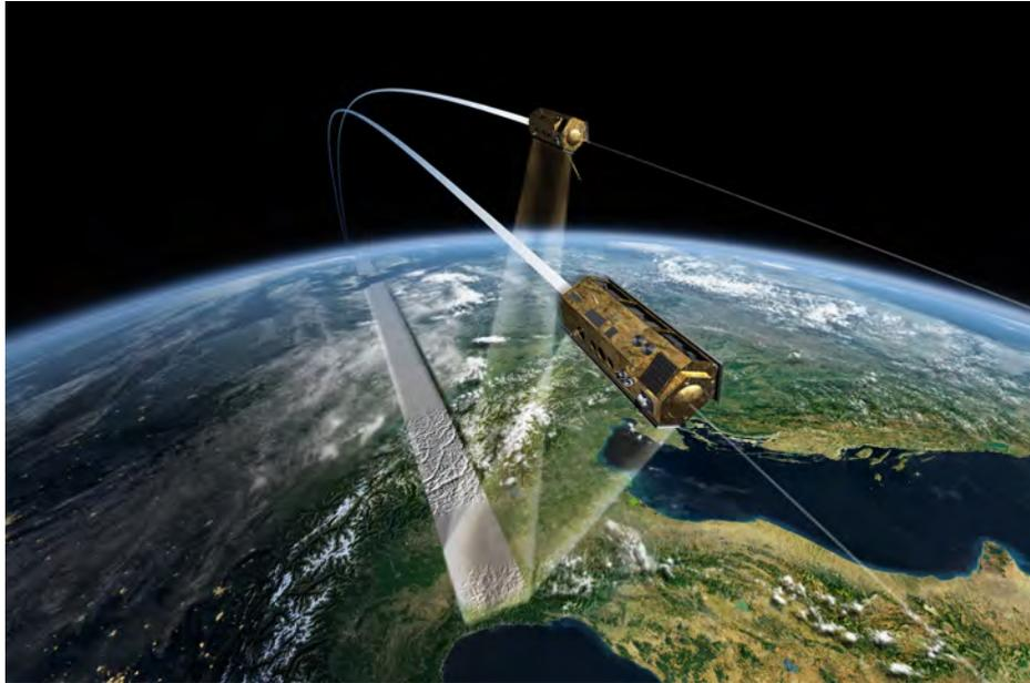
**Figure 1.3:** TanDem-X spacecraft formation. Courtesy of DLR.
