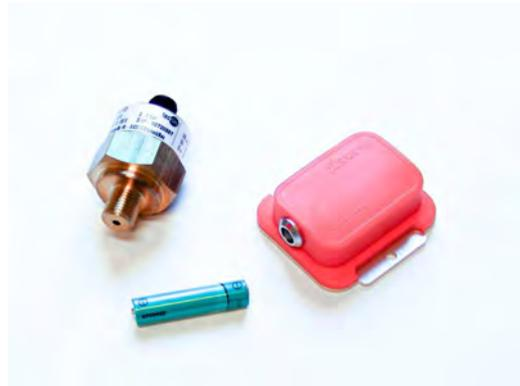
(b) Tecsis pressure sensor and XSens IMU. The battery is of size AAA
