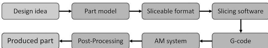
Figure 10.6 Typical pipeline for an AM process.
