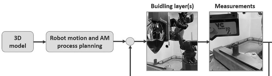
Figure 10.13 The concept of feedback control in AM processes.
