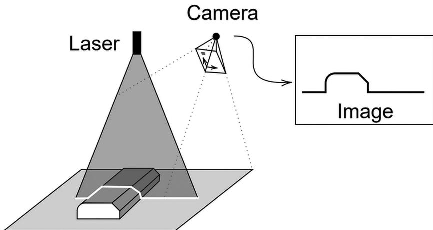
Figure 10.11 Working principle of line laser scanners.
