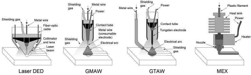
Figure 10.1 Schematic drawings for several AM processes.
