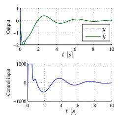
Fig. 3. Closed-loop performance with r=2 and an optimized basis. Top: High-fidelity y and estimated  $\hat{y}$ . Bottom: eMPC control input, constrained such that |u|<1000. The input constraint is seen to be active during the first half second.
