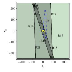
Fig. 4. Example of state-space partition for a reduced-order model with r=2, with state trajectory starting in o and ending in \*. The different color shades indicate the 21 regions  $\mathbf{R}_i$  in the state space. The controller feedback matrices  $(K_i,k_i)$  are constant within each region.
