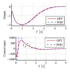
Fig. 5. Performance comparison for r=5 with eMPC horizon N=10. Top: Output of the full model using reduced-order control based on optimized- and POD basis. Bottom: Control input for the two different cases.
