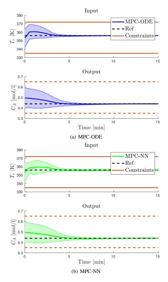
Fig. 3: Results from 100 simulations. The thick line represents the emperical mean, and the shaded area represents  $\pm \sigma$ . In each figure, the upper subplot shows the coolant temperature reference and the bottom subplot shows the concentration. Note that the input constraints are hard, while the output constraints are soft.
