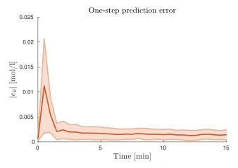
Fig. 4: The one-step prediction error for the prediction model used by the MPC-NN. The thick line represents the empirical mean, and the shaded area represents  $\pm \sigma$  from 100 simulations.
