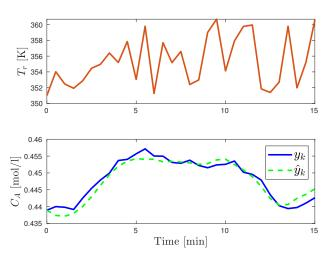
Fig. 2: Top: random steps in the coolant temperature reference. Bottom: true and multi-step ahead predictions of the concentration, with the network in parallel mode, using a separate validation set not previously seen by the network. The output is shown in original scale. The multi-step ahead prediction seems to be fairly accurate for a random input sequence, and for that reason more complex and larger architectures are avoided in order to keep the prediction model simple.
