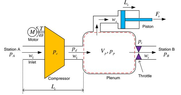
FIGURE 3. Compression system equipped with combined active surge control system and surge avoidance system.
