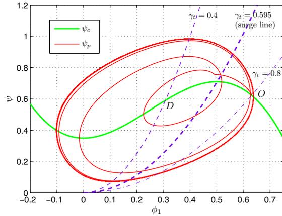
**FIGURE 8.** System trajectory of compressor with PAASCS when the piston is saturated.
