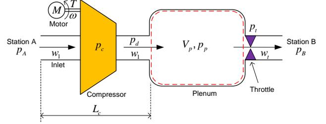
**FIGURE 1.** Model of basic compression system.
